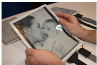
A collaboration between eReader maker Plastic Logic, Intel and the Queen's University Human Media Lab, the PaperTab is a 10.7-inch prototype running on a Core i5 processor with a black and white display.
