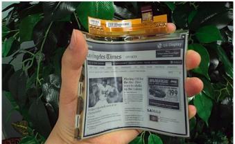
The LG design measures 6" diagonally and handles XGA (1024x768) resolutions. Construction is in plastic, meaning the display is only 0.7mm thick and weighs 14g (50% less than traditional glass displays). It is not able to handle colours or animation, but should offer a crisp reading experience.
