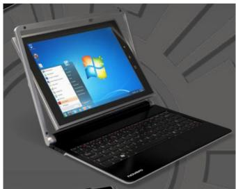
The flip-rotating design allows users to switch between notebook and tablet modes, while double-clicking a shortcut switches between operating systems. The device was first seen at the Intel CES 2012 as a prototype.
