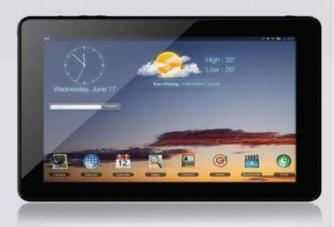
It carries a 10.1" capacitative LED backlit TFT LCD touchscreen with 1280x800 resolution.
