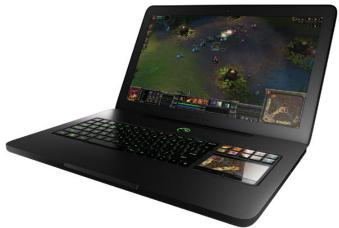
It comes in a portable package-- 22.5mm thick and weighing 3.2kg-- with a 17" display, 2.8GHz i7 processor, 8GB RAM, 320GB SATA HDD and a GeForce GT555M video card.
