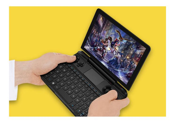
Like other machines in the GDP Win series, the Win Max is a Windows 10 laptop with built-in gaming controls, namely a pair of clickable analogue sticks, d-pad, four face buttons and shoulder triggers. It also features an 8-inch 1280 x 800 resolution touchscreen able to push up to 500 nits brightness with 90% of the DCI-P3 colour gamut, while the miniature keyboard is backlit and includes a touchpad.
