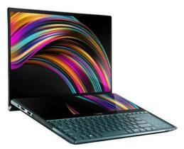
The second display is set directly above the keyboard, and is the same width and half the width as the main display. In other words it is something of an overpowered MacBook Pro Touch Bar, since it is touch-enabled and allows for dedicated shortcuts and function buttons for specific apps. It also doubles as either a regular display or even two, since users can split it into two small 16:9 windows.
