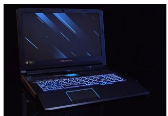
Acer calls it the keyboard "HyperDrift," and says the mechanism allows for improved cooling and performance. The keyboard slides towards the user, making for an admittedly bulky device, even if it adds an ergonomic wrist rest. Furthermore, the keyboard includes MagForce switches on the WASD keys for "analog-like" control, as well as per-key RGB lighting and a Turbo hotkey to overclock the CPU.
