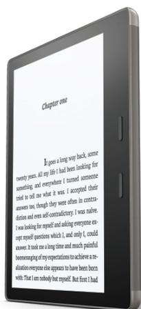
The Kindle Oasis has a 300ppi 7inch display equipped with 12 LEDs for more uniform front lighting. Ambient light sensors tweak the lighting according to the environment, and the display is covered with a proprietary glass Amazon says is its toughest yet. A built-in accelerometer automatically switches page orientation according to how the eReader is held.
