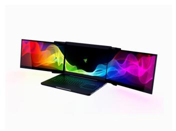
For the full triple-display experience one needs to slide two full-size screens from the size of the main monitor, creating a crazy widescreen display. The displays are top-notch, being 4K IGZO panels complete with Nvidia G-Sync and Surround technologies to ensure immersive multi-display action in 12K resolution.
