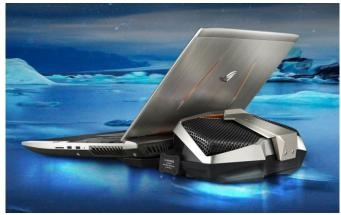
The GX800 is a super-sized gaming laptop, with an 18.4-inch 3840 x 2160 resolution display promising to cover 100% of RGB colour space. Inside is an Intel Core i7-6820HK CPU, a 45W TDP 4C/8T number normally running at 2.7/3.6GHz. However, the addition of the grandly named Hydro Overclocking System boosts the clock to 4.2GHz, while the DDR4 RAM inside the machine gets clocked as high as 2800MHz.
