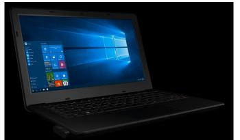
Each mini-PC module is a self-contained Windows 10 PC, and the concept behind the Kangaroo Notebook has users switching between different modules dedicated to different uses. In fact, InFocus insists on the concept so much the package contains 2 modules, each featuring Windows 10, an Intel Z8350 Cherry Trail CPU, 2GB RAM and 32GB storage together with the laptop dock.
