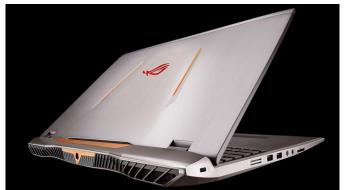
As such, the G701 lacks the cooling required for overclocking duties, but still offers some tweaking options through ROG Gaming Centre software. It is also described as a VR-ready machine, as it carries an Intel i7 6820HK CPU, GeForce GTX 980 GPU, 8 to 64GB of DDR4 RAM and either dual-512 or 256GB SSDs in RAID 0 configuration (no ODD).
