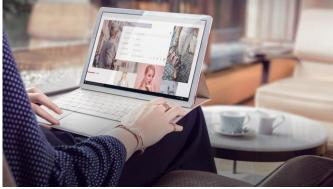
Weighing 640g and being 6.9mm thick, the MateBook carries a 6th gen Intel Core M CPU (ranges up to 3.1GHz), 4/8GB RAM and 128/256/512GB SSD. The 12-inch IPS LCD handles 2160x1440 resolution, the battery promises to power 9 hours of video playback (or 13 hour of lighter use) and the device should remain cool during use via heat dissipation technology.
