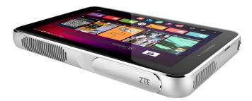
Announced at MWC 2016, the Spro Plus combines a 500 lumen projector with a Snapdragon 801 CPU, 3GB RAM, 128GB storage (expandable via SDXC card) and 12100mAh battery. Connectivity comes through wifi, Bluetooth and optional LTE. As such, one can easily describe it as a chunky mid-range tablet able to beam 80-inch images on walls or screens.
