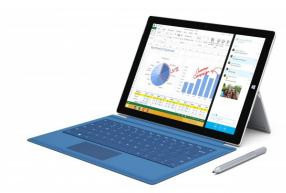
In fact the Surface Pro 3 is 12-inch device, up from the 10.6-inch of the previous model, with a 2160 x 1440 ClearType display. It is also relatively slim (7.6mm) and light (800g), at least when compared with ultralight laptops. Such comparisons are apt, since Microsoft itself describes the device as a "revolutionary laptop" (not "iPad killer") when paired with the companion Type Cover keyboard/cover.
