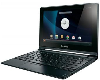
It runs on Android 4.2, weighs 1kg, is 17.3mm thick and is designed for both entertainment and productivity applications. Inside are a 1.6GHz quad-core Cortex-A9 processor and a battery promising up to 9 hours of continuous video playback.
