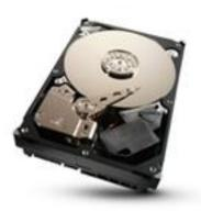
Seagate unveils what it calls the world's first 3.5" HDD with 1TB of storage per disk platter-taking Samsung's 625 Gigabits per square inch technology and putting it in an actual product.
