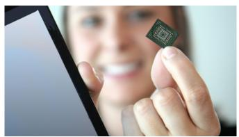
SanDisk and Toshiba's developments in NAND flash memory get even smaller-- producing a 64Gb X2-based monolithic chip with 19nm technology.
