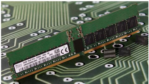
The company first detailed its DDR5 plan <u>s back in February 2019</u> with the presentation of a DDR5-6400 memory chip at the International Solid State Circuits Conference. The technology offers two times the bandwidth compared to DDR4, with the aim of reaching over 4800Mbps, allowing it to handle the demands of massively multi-core CPUs.
