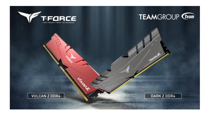
Aimed at gamers on both Intel and AMD platforms, the memory kits feature angular aluminium heatspreaders in red or gray, but lack the RGB LEDs typical of similar products. The Vulkan Z heatspreaders measure 32 x 140 x 7mm, and are available in both dual-channel (32GB x2) and single kits, with a choice between DDR4-2666MHz CL18-18-18-43 1.2V and DDR4-3000MHz CL16-18-18-38 1.35V modules.
