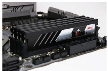
The Evo Spear Phantom Gaming memory modules come in DDR4-2400, DDR4-2666, DDR4-3000 and DDR4-3200 versions, with latencies ranging from CL17-19. The lower end modules run at voltages of 1.2V, while the higher-spec modules run at 1.35V. The kits also include an XMP 2.0 profule for one-click overclocking, and individual stick capacity reaches up to 16GB.
