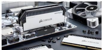
Further enhancing the look of the memory modules are white LEDs on top bar bearing the "Dominator" branding. On the inside is "industry leading 10-layer PCB and patented DHX cooling technology," together with "carefully screened and selected Samsung ICs." Being premium modules, these are "engineered for world-class system builds" and "meticulously designed with painstaking attention to detail."
