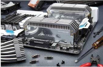
Designed for systems based on Intel X99 and 100 series motherboards, the modules are clocked at 3200MHz and can be overclocked to 3600MHz. Also included is a 10-lyaer PCB, DHX cooling and full XMP certification for one-touch overclocking. However what makes the modules a "Special Edition" is looks, with a choice of either "Chrome" polished or "Blackout" matte finishes.
