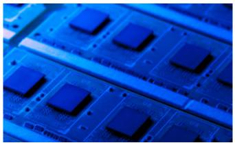
Innodisk launches a memory module range equipped with conformal coatings to provide protection against moisture, dust and chemical contaminants, thus allowing normal operation even in extreme environments.
