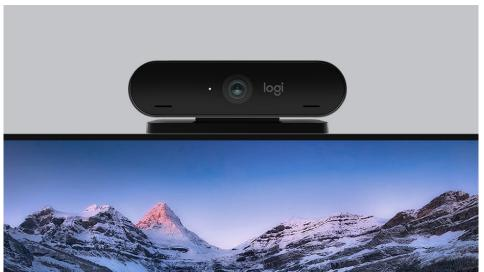
The 4K Pro Magnetic Webcam attaches to the display using a specially designed stand and a magnet Logitech claims remains attached even when users rotate the display into portrait mode. It should even automatically rotate video input in case the display is rotated, meaning users can video chat no matter the orientation of the monitor.
