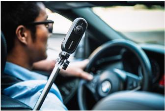
The One is a small device the size of a small sausage link. It features 2 cameras, and can either be plugged into the iPhone Lightning port or used remotely, with the phone acting as Bluetooth controller. Gyroscopic stabilisation promises more steady video recording, the main body has a built-in tripod mount and an included protective case doubles as a stand.
