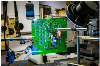
According to the researchers, the OPA does what lenses do-- manipulate incoming light-computationally instead of optically. Whereas lenses bend incoming light to focus it on a piece of film or an optical sensor, the OPA uses an array of light receivers to add a tightly controlled time delay (or phase shift) to the light. This allows the camera to selectively "look" in different directions, and focus on different objects.
