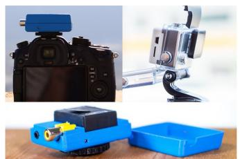
The SteadXP is essentially a small box containing a 3-axis accelerometer and gyroscope, as well as 32-bit ARM processor, microSD card slot and USB connectivity. It records the motion data of the shot in question in order to build a smooth, steadicam-style version.
