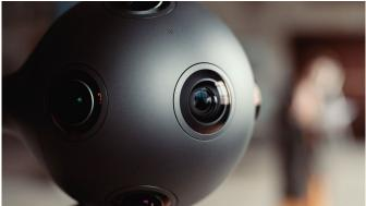
A creation of the Nokia Technologies division, the Ozo looks a bit like a Star Wars prop. It captures 360-degree video through 8 synchronised shutter sensors, and carries 8 integrated audio for the recording of surround audio. Meanwhile built-in software allows real-time viewing of shot footage through regular VR headsets, bypassing the need to pre-assemble panoramic images.
