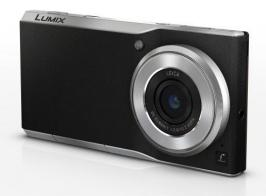
Revealed at Photokina 2014, the CM1 is the first device of its hybrid ilk to carry a 1-inch 20MP CMOS sensor together with f/2.8 Leica optics, mechanical shutter and a manual control ring. It also looks unlike any other smartphone on the market, with retro-style silver metal and mate black casing similar to those of, well, cameras.
