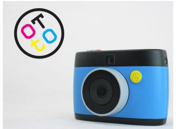
Essentially a Raspberry Pi microcomputer and a lens inside a disposable camera-style case, the Otto features a rotating crank next to the regular shutter button. Capturing an animated picture simply involves rewinding the crank by one turn, before an app syncs the recording as an animated gif on smartphones.
