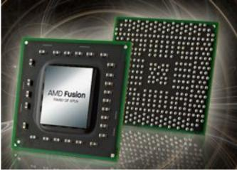
These APUs incorporate – in a single die design – multi-core CPU (x86) technology, a discrete-level graphics and parallel processing engine for DirectX 11, a dedicated high-def video acceleration block, and a high-speed bus (speeds data across the differing types of processor cores within the design).
