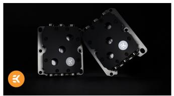
The water blocks feature a machined copper base treated with nickel electroplating. The top is made of black POM acetal, while the hold-down brackets are in stainless steel. A total of 9 water ports (x3 standard G1/4" ports on top and x6 G1/8" threaded ports on the sides) allows compatibility with both taller and lower-profile cooling solutions.
