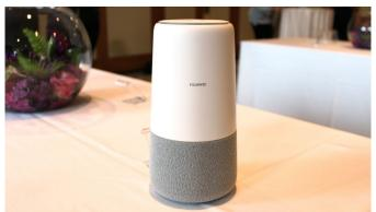
The result of a Huawei-Amazon collaboration presented at IFA 2018, the AI Cube runs on Alexa and promises a more convenient way to both connect to the internet and control smart devices. A slot for an LTE SIM card makes it a 4G hot spot, while an ethernet port allows use as an 802.11ac wifi router. The router is dual-band, working on the 2.4 and 5GHz bands, and transmits data over LAN at up to 1200Mbps.
