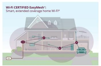
As the organisation puts it, EasyMesh will provide customers and service providers with a selection of interoperable devices across difference brands to ensure wide and reliable wifi coverage. The technology coordinates multiple access points into a "unified and intelligent" wifi network able to autonomously aid all areas of the home for complete coverage.
