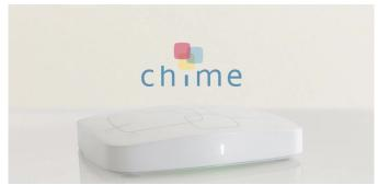
Like other mesh network routers found in enterprise environments, multiple Chime units work together to cover the house in "strong and reliable" wifi. The 802.11ac router features dual-band 2.4/5GHz radios, together with a dual-core CPU, x1 USB 2.0 port and x2 ethernet port, and AVG claims a single Chime handles up to 50 devices.
