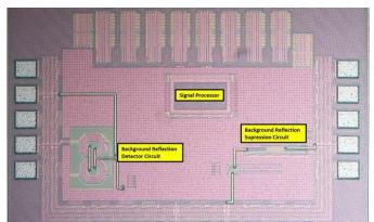
"The idea is if the wearable device only needs to reflect the wifi signal from a router or cell tower, instead of generate it, the power consumption can go way down (and the battery life can go way up)," researcher Adrian Tang says.
