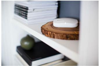
The Eero amounts to a router, wireless access point and range extender inside a small, white box. It features dual-wifi radios for simultaneous 2.4 and 5GHz connections, 802.11a/b/ac support and built-in Bluetooth 4.0, and according to the company provides up to 1000 square feet (around 92 square metres) of 50-100mbps wifi coverage. Thus the average house requires multiple Eeros, which is where the makers claim cleverness as the routers pair automatically to form an instant mesh network.
