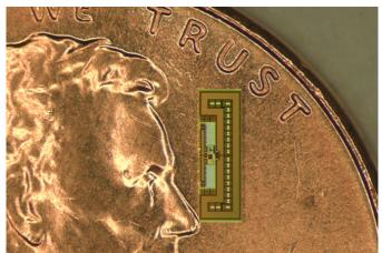
Similar tiny radios already exist, but unlike similar solutions (which operate on low frequencies), the Berkeley/Stanford radio receives data on the 24GHz band and transmits on 60GHz. This reduces the power requirements by so much the radio charges itself with energy from received signals.
