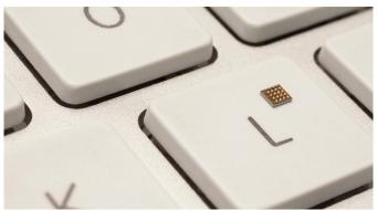
The KL02 measures all of 1.9 x 2.0mm and still is a full MCU, with 32k of flash memory, 4K RAM, 32-bit 48MHz ARM Cortex-MO+ processor and built-in autonomous peripherals (including a 12-bit analog-to-digital converter and a low-power UART) allowing device makers to build increasingly smaller boards for tiny devices.
