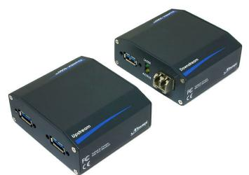
Shown at a press event at CES 2012, the FireNEX-uLINK-D is bus powered (needing no external power or drivers) and plug and play.
