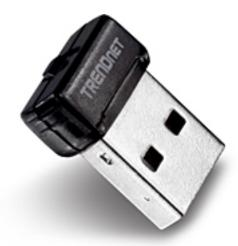
The adapter is ideal for laptops. Once plugged into USB port the adapter extends only 0.8cm from the machine's edge.
