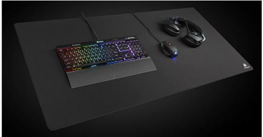
Built for "maximum durability," the Scimitar RGB Elite has a sturdy scroll wheel, 1.8m braided cable and Omron switches rated for 50 million clicks. The left side houses 12 of the 17 buttons, as arranged in a sculpted and textured 3x4 array. Users can program the buttons for custom macros and button remaps, as well as as adjust their position by 8mm via "Key Slider control system" in order to accommodate for different size hands.
