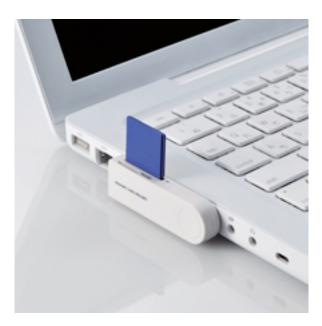
The device doesn't stick out perpendicularly to the machine's side, but lays flat on the side. It also swivels as needed, getting out of the way if it covers up other ports next to it.
