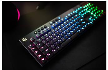
GL switches come in 3 variants, linear, tacticle and clicky, or the equivalent of the Cherry MX Red, Brown and Blue switches. Logitech claims they are 50% the height of standard mechnical switches and offer 25% faster presses, making for a more comfortable typing experience.
