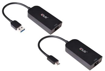
The CAC-1420 (USB-A to 2.5 GbE) and CAC-1520 (USB-C to 2.5 GbE) are exactly what it says on the tin. They feature an RJ-45 connector on one side and a USB 3.1 interface on the other, and are compatible with Windows 8/10 PCs and Macs running on OS X 10.6 to 10.14. Being USB-powered no external power adapter is required.
