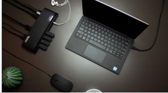
The docking station supports two extra displays of either the HDMI or DisplayPort variety, while adding x6 USB 3.0 ports, ethernet and audio ports to connect any device to the laptop. Compatible with Windows PCs and laptops, it offers x2 HDMI and x2 DisplayPort outputs for mirroring or extending a desktop to up to two external monitors.
