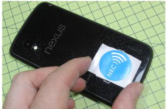
The WLC enables a single antenna in the NFC-enabled device to manage both communications and charging. Such a solution should allow for easier charging of low-power IoT devices, such as smartwatches, fitness trackers, headsets and other consumer devices. It uses the 13.56MHz base frequency, and leverages the NFC communication link to control power transfer.
