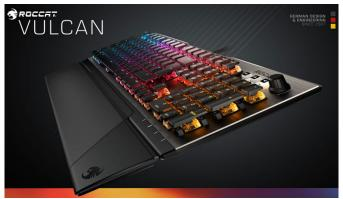
The Titan switch is supposedly designed "from the ground up" for gamer customers, with a tactile 1.8mm actuation point, 3.6mm travel distance and quiet performance. The result, the company claims, is "the most responsive and best-feeling key stroke ever," especially when combined with the ultra-light key caps (50% than standard) found in the Vulcan keyboard.
